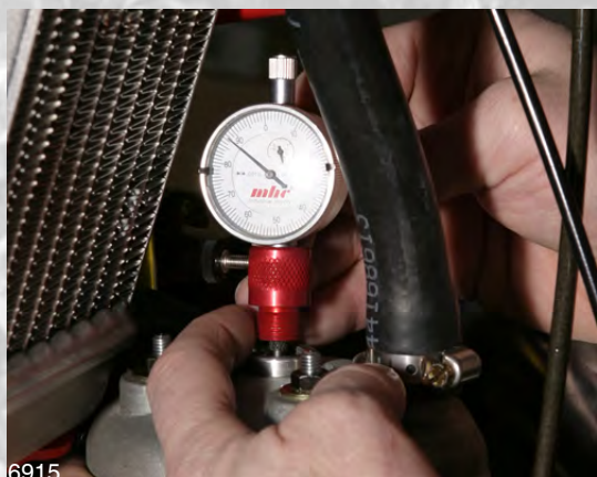
3. Insert Dial Indicator (Cobra part # ECMU0079) into spark plug hole.
