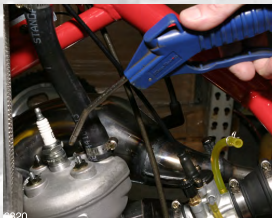
1. Clean debris from around spark plug area to make sure no foreign objects fall into cylinder.
