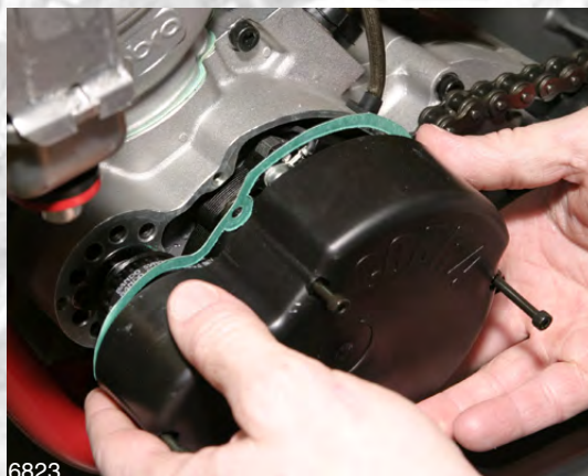
6. Remove the stator cover from the engine being careful not to tear the stator cover gasket during disassembly.
