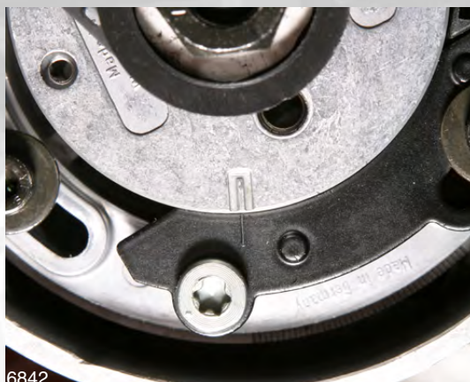
12. Now check to see if the line on your stator and the line on your rotor are lined up directly.
