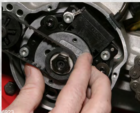
11. Next turn the crankshaft clockwise until the dial indicator reaches 0.040 (1.02mm) Before Top Dead Center (BTDC) or your desired setting. *See note at bottom of page.
