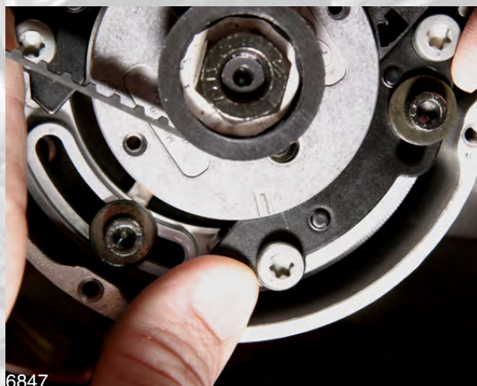
14. After stator assembly is loosened up you will need to adjust the stator plate in the proper direction required to line up your timing mark lines.
