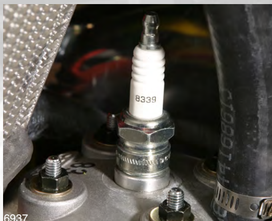
19. Install Champion 8339 Spark plug using 13/16 wrench.
