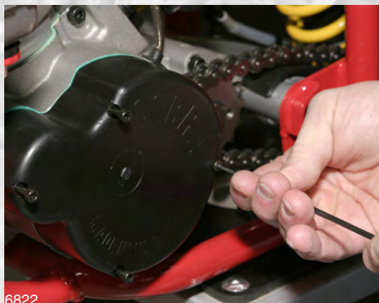
5. Remove the four socket head bolts from the ignition cover using a 3mm Allen wrench.
