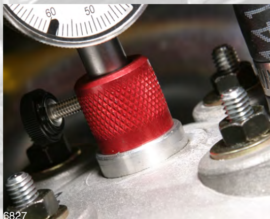
4. Make sure dial indicator collar is tightened down snugly to cylinder head insert. A loose fit here can cause your timing to be off.
