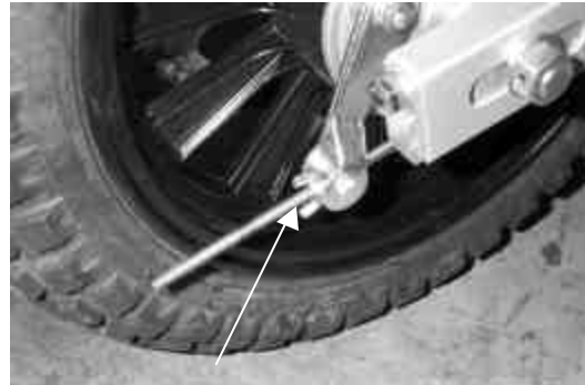
Figure 7 , adjust lever 'free play'
